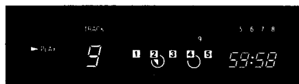
d. Total time of the disc (number of tracks is also displayed).
